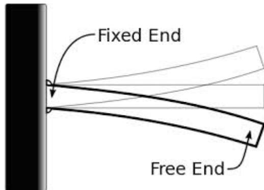
A **cantilever beam** is supported on one end with a fixed support, and free on the other end
