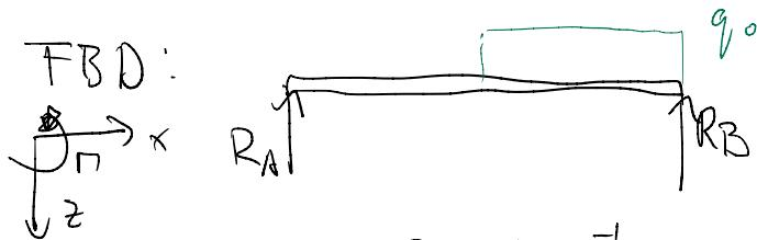
$$q(x) = -R_A \langle x \rangle^1 + q_0 \langle x - \frac{L}{2} \rangle^0 - R_B \langle x - L \rangle^1$$
