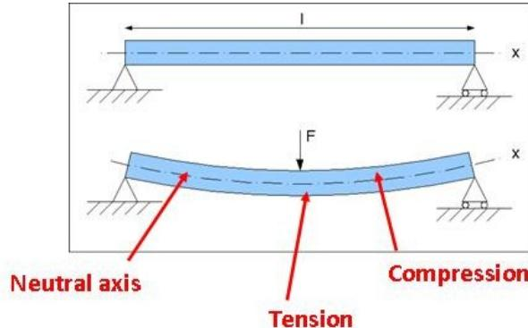
A **simply supported beam** is supported on one end with a pin support, on the other with a roller support.
